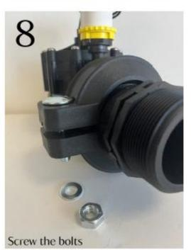
For an easiest assembly you can lubricate the gasket with silicone grease
